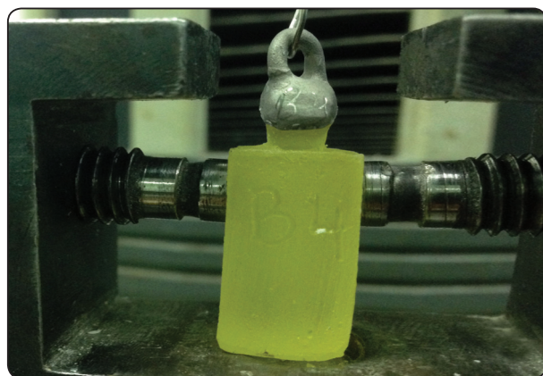
FIG. (7) Sample during tensile testing.
