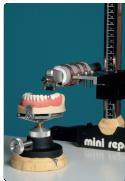
Fig. (2) Proximal contact measurements by tooth pressure meter
