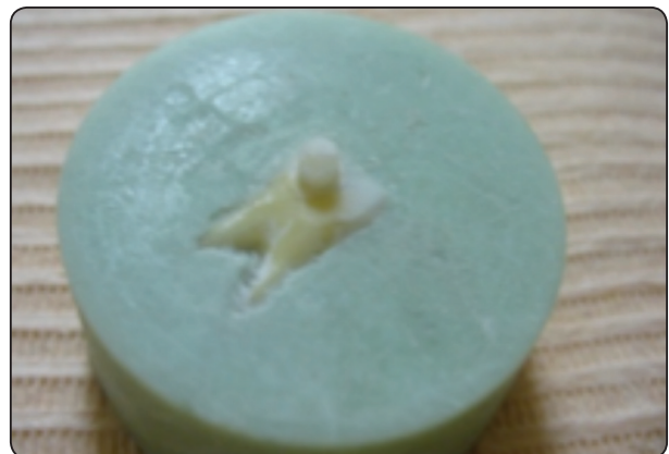
Fig. (1) Specially designed splitted Teflon ring used to create composite cylinders to tooth samples
